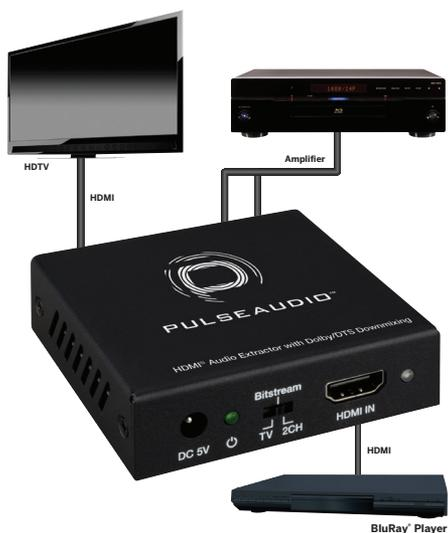
1. Connect an HDMI source to the HDMI input
