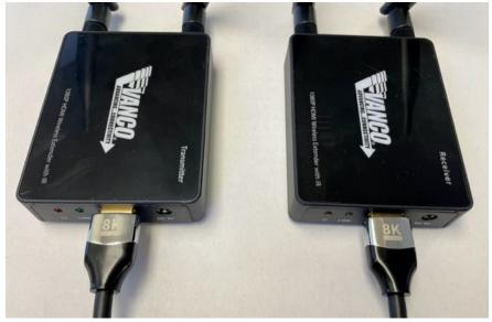
2. Power on the receiver. The POWER LED and LINK LED of the receiver will be on and solid.
