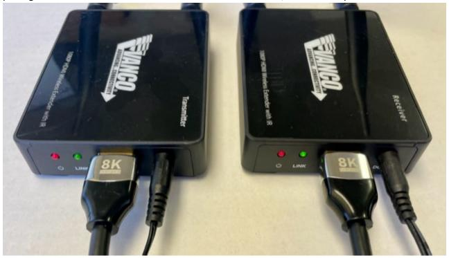
NOTE: The LINK LED on the receiver will always be on through the pairing process.
