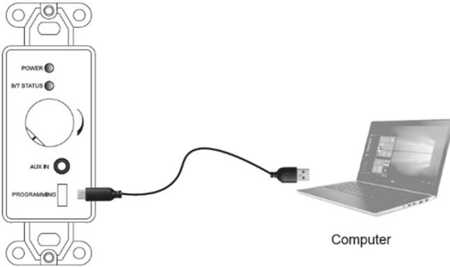
1. Connect a Micro USB Cable from the PA230BWA to a computer's USB port
