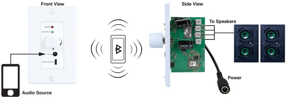
NOTE: Ensure all speaker(s) and power wires are run in accordance with local laws and regulations. Before inserting the amplifier into the electrical box and wall, either note or remove the Bluetooth password found on the sticker on the back of the unit.
