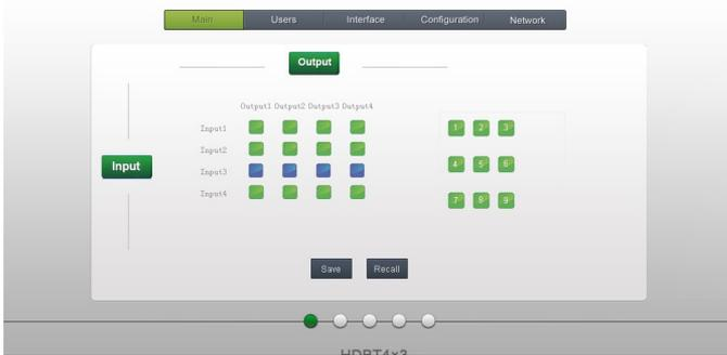
The button matrix displays every possible connection between every input and output, users can carry on the connections by clicking corresponding button.
