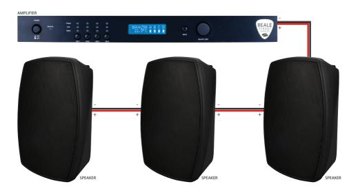
The total number of speakers multiplied by the tap value cannot exceed the output power (in watts) of the 70V/100V amplifer. The example below shows 3 total speakers. Using the 10W taps, you will need an amplifer with at least 30W (3 speakers x 10W tap).
