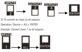
Note: Indicators of the pressed buttons will blink green for three times if the conversion is done, then it will be off. If the conversion failed, they will be off immediately.
