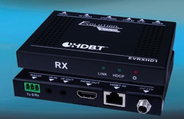
Features POC (Power over Cable) technology, providing power for the receivers
