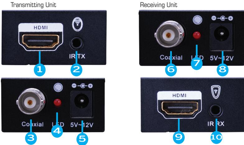
1. HDMI: Connect the HDMI source with an HDMI cable.
