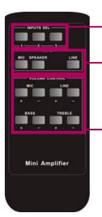
Input Selection - Choose between up to 3 inputs connected to the PAV140 Input 1: Dual RCA audio input Input 2: 3.5mm audio input Input 3: Optical Digital audio input Mute Function - Mute and unmute inputs, outputs, and/or MIC volume
