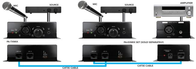
To add additional sources, the PA-EXMIX allows for cascading additional PA-TXMIX Transmitters (sold separately). See below for connecting an additional Transmitter:
