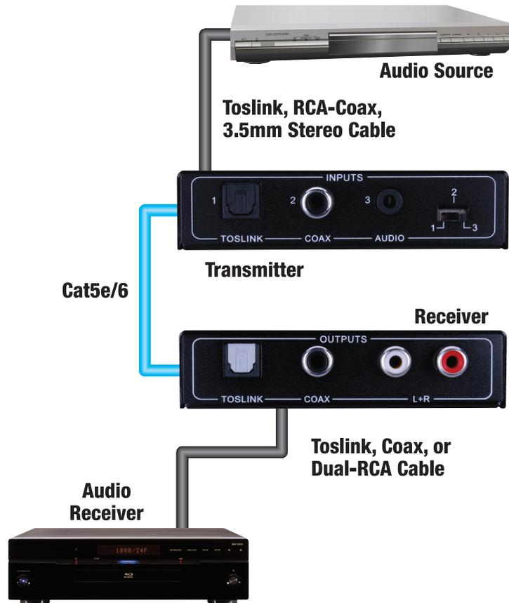
Analog audio extension over a single Cat5e/6 via 3.5mm connection
