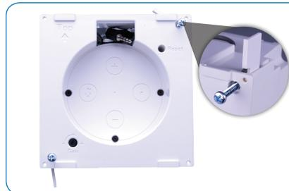
7. Mount the **Spot For Dot** into the wall using the screws and wing clamps. Tighten both screws until the **Spot For Dot** is secure and flush with the drywall.
