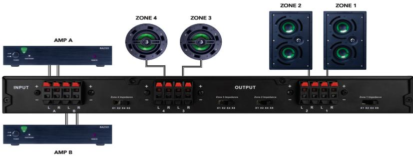
1. With any and all amplifiers and sources turned off, connect the speaker wire to the appropriate “+/-” terminals of each speaker
