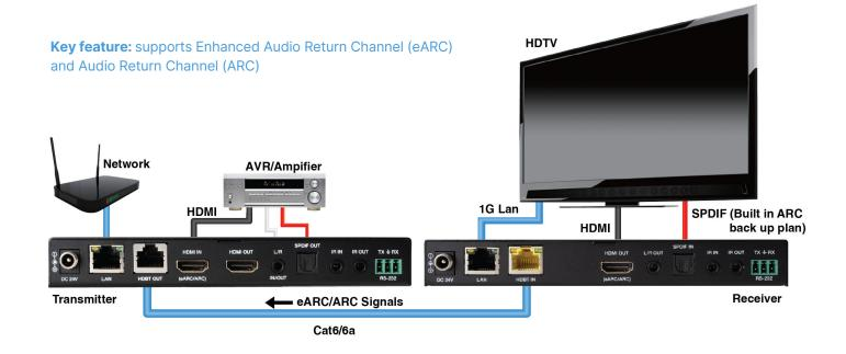
The Evolution by Vanco EVEXHDB3 HDBaseT 3.0 extender offers multiple options for pass-through control, and audio including eARC and ARC, along with PoH while being able to extend uncompressed 4K with HDR up to 164ft/50m over a single Cat6 or up to 328ft/100m using Cat6a/7.
