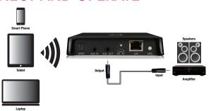
The PASTREAM2 Receiver is a device that receives internet streaming music or other wireless music from any wifi enabled device. Multiple PASTREAM devices such as the PASTREAM2 and PA230SWA (sold separately) receivers can be used in a single distributed audio system to create multiple streaming sources.
