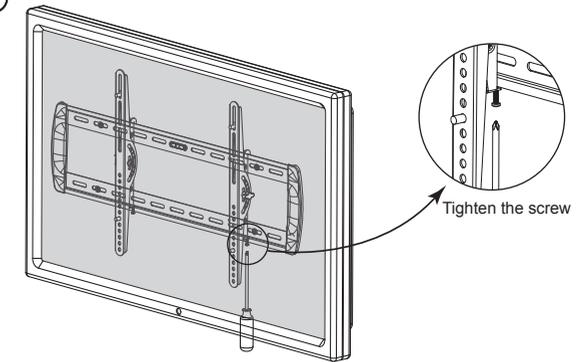
The lock designed feature can prevent your television being removed from the panel.
