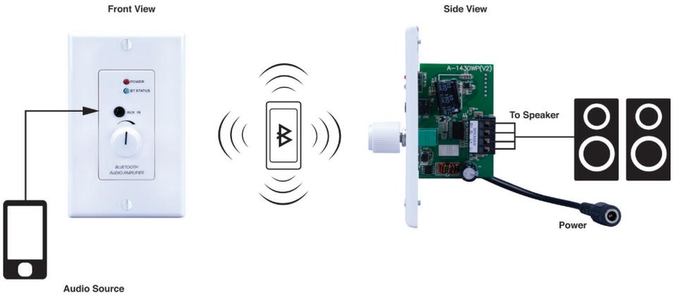
NOTE: Ensure all speaker and power wires are run in accordance to local laws and regulations. Before inserting the amplifier into the electrical box and wall, either note or remove the Bluetooth password found on the sticker of the back of the unit.
